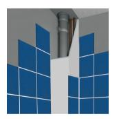
Smooth, paintable pipe covers are a quick and effective solution for hiding away unsightly pipework, simply choose the correct cover size and cut to length. Run a bead of Nicobond PU Adhesive along the 2 leading edges and press firmly into position.
